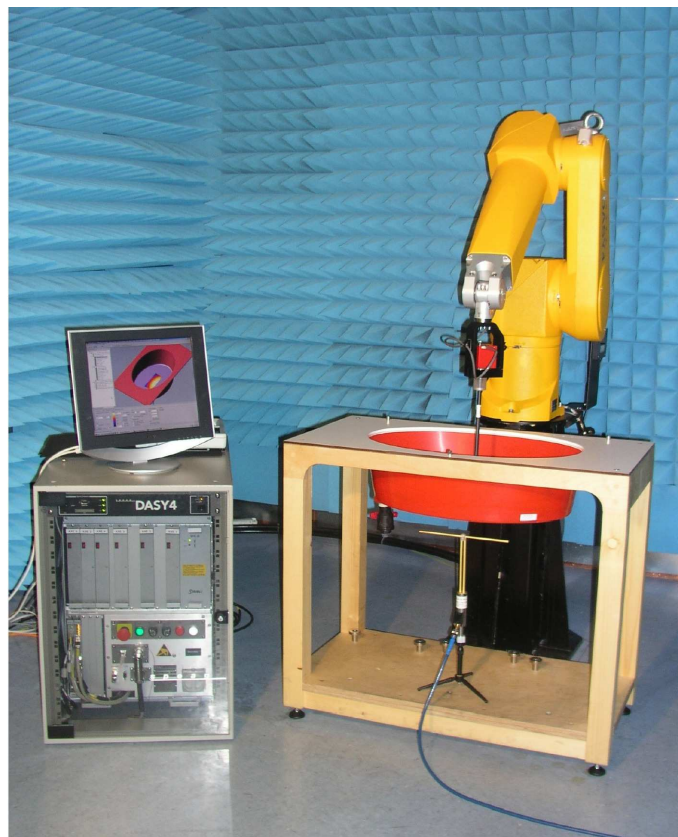
Figure 1: DASY 4 dosimetric assessment system (SPEAG)
