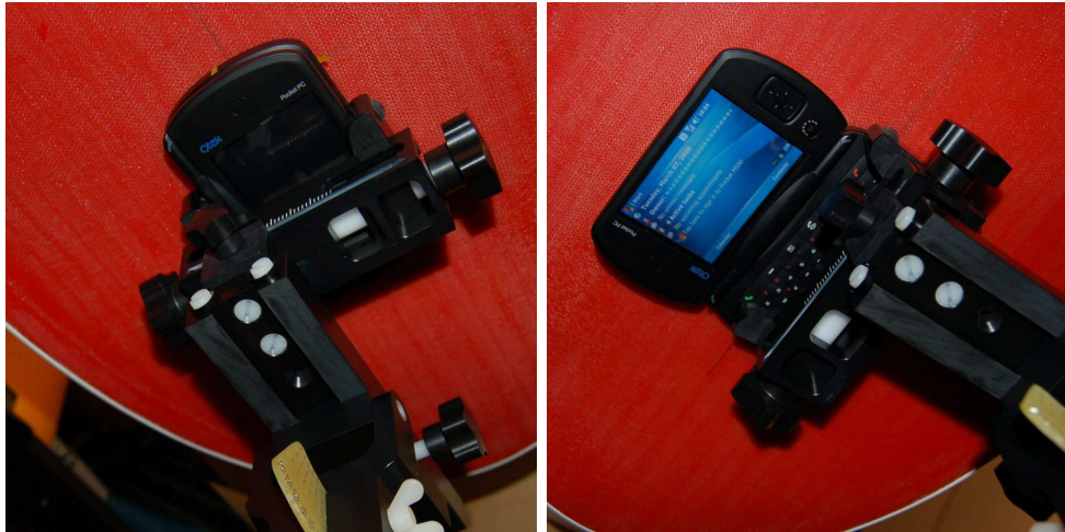
(a) QTEK 9000 in PDA mode attached to the phantom (b) QTEK 9000 in Laptop mode (display 180°) attached to the phantom
