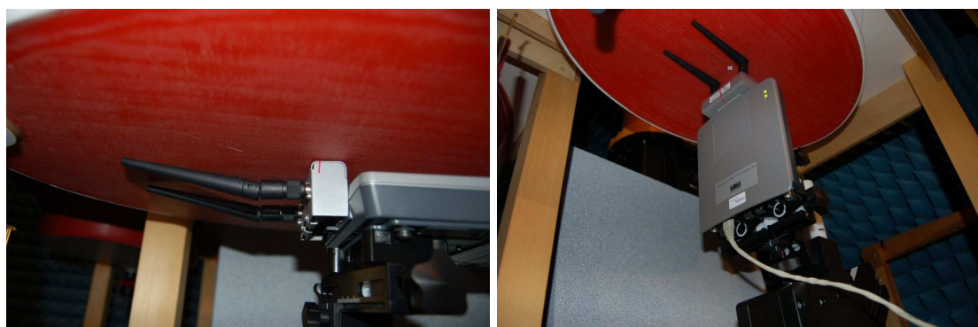
(a) Aironet 1200 Root Bridge and Non Root Bridge in flat orientation (IEEE802.11a) (b) Aironet 1200 Root Bridge and Non Root Bridge in perpendicular orientation (worst-case) (IEEE802.11a)
