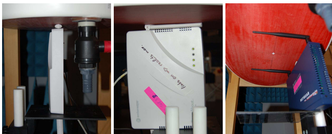
(c) Enterasys Roamabout RBT-4102 worst-case orientation (IEEE802.11a/b/g) (d) Netgear ProSafe WG302 802.11g worst case orientation (IEEE802.11b/g)
