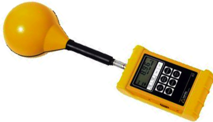
Figure 12: Narda exposure level tester ELT-400.
