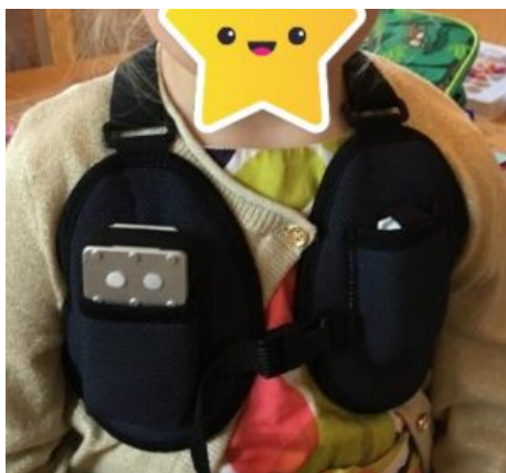
Figure 1: Image of a child wearing the strap containing the two dosimeters. The UV dosimeter is on the left, with the two sensors that measure UVA and UVB radiation.
